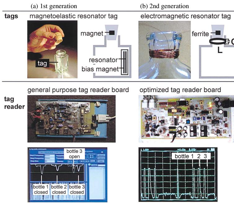
**Fig. 9** Wireless sensing technologies.
