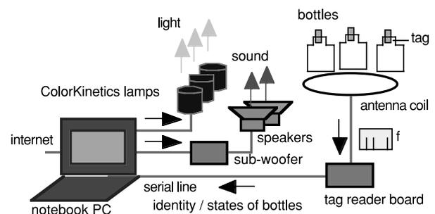
Fig. 2 System configuration of the bottles.
